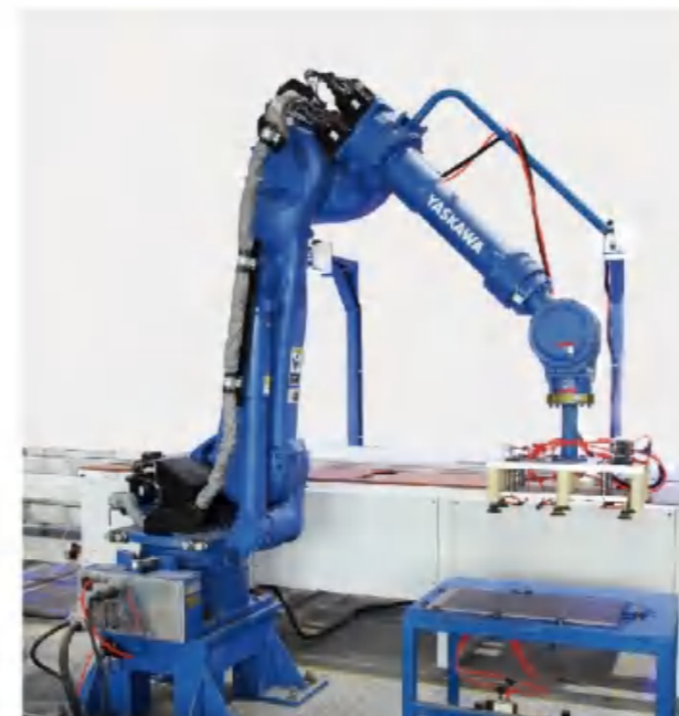
Industrial robot (automatic tile placement)
